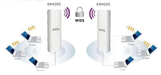
Not every Access Point device has support WDS in Access Point Mode. It is recommended using ENH202 if you would like to use this service.
