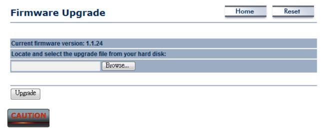
Upgrade process may take few minutes, please do not power off the device and it may cause the device crashed or unusable. ENH202 will restart automatically once the upgrade is completed.
